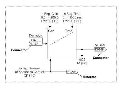
Connectors and binectors are identified by a name and number. Connectors with 16 bit resolution are identified with a "K". Connectors with 32 bit resolution are identified with a "KK". Binectors are identified with a "B".
