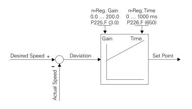
The PI-controller's job is to make speed corrections quickly a minimal amount of overshoot and oscillation. Parameter P225 (gain) and parameter P226 (time) are used to tune the PI-controller's performance. The end result should be a fast response time with about a 43% initial overshoot. The motor should then settle in to the new desired speed.
